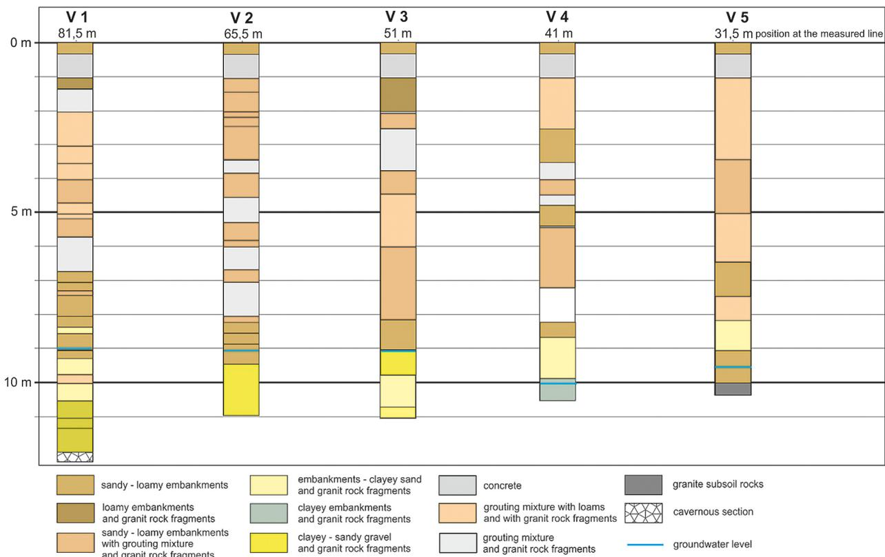
Fig. 1. Logs of wells V1 – V5 interpreted based on the drilled cores.
