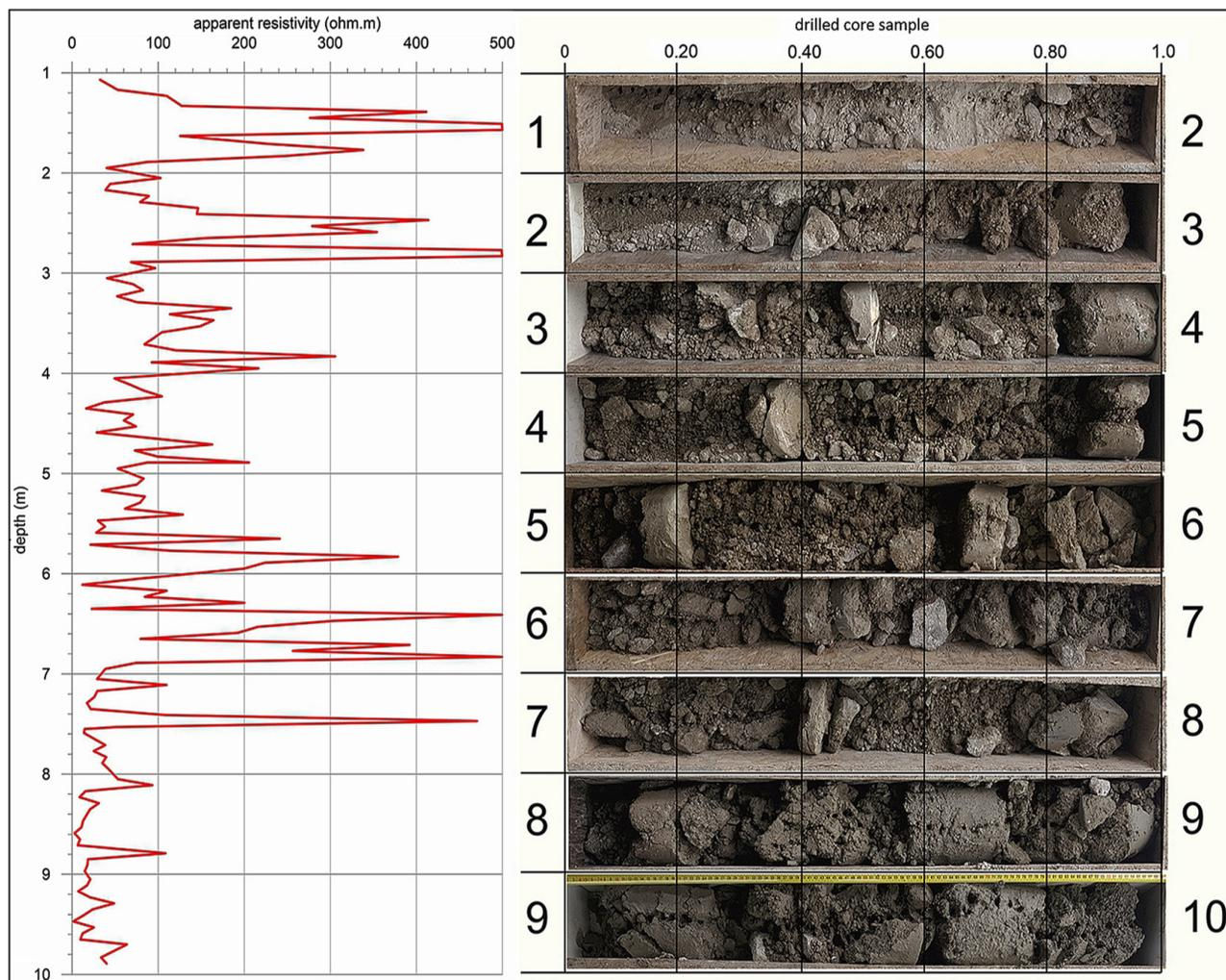
Fig. 3. The result of electrical resistivity measurement on the core sample; left - measured resistivity, right - drilled core sample.
