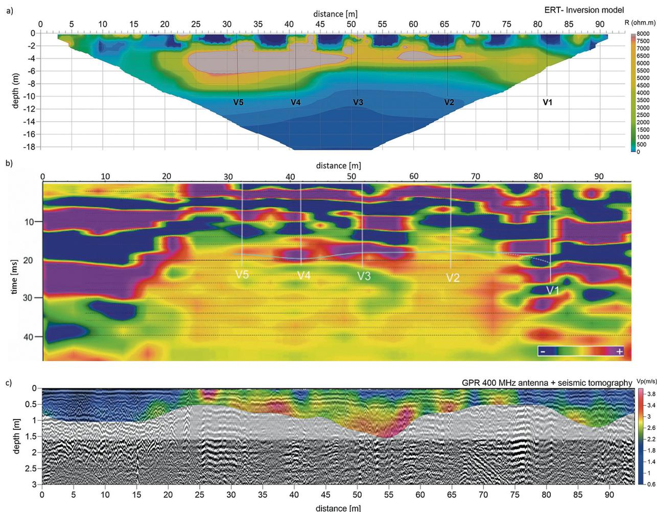
Fig. 4. The results of geophysical measurements: a) inverse resistivity profile ERT with position of wells, b) seismic reflection profile (time profile with wells position, c) combined results of GPR measurement and SRT measurements.
