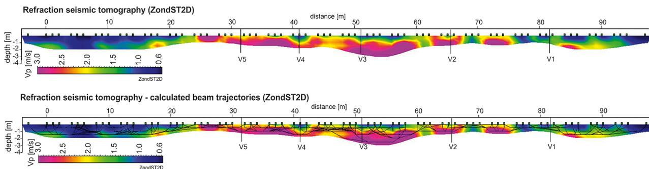
Fig. 5. Final velocity model of the seismic refraction tomography.
